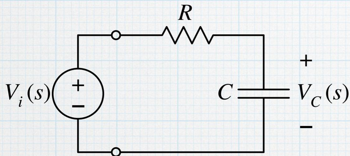
$$V_C(s) = \left( \frac{\frac{1}{RC}}{s + \frac{1}{RC}} \right) V_i(s)$$
