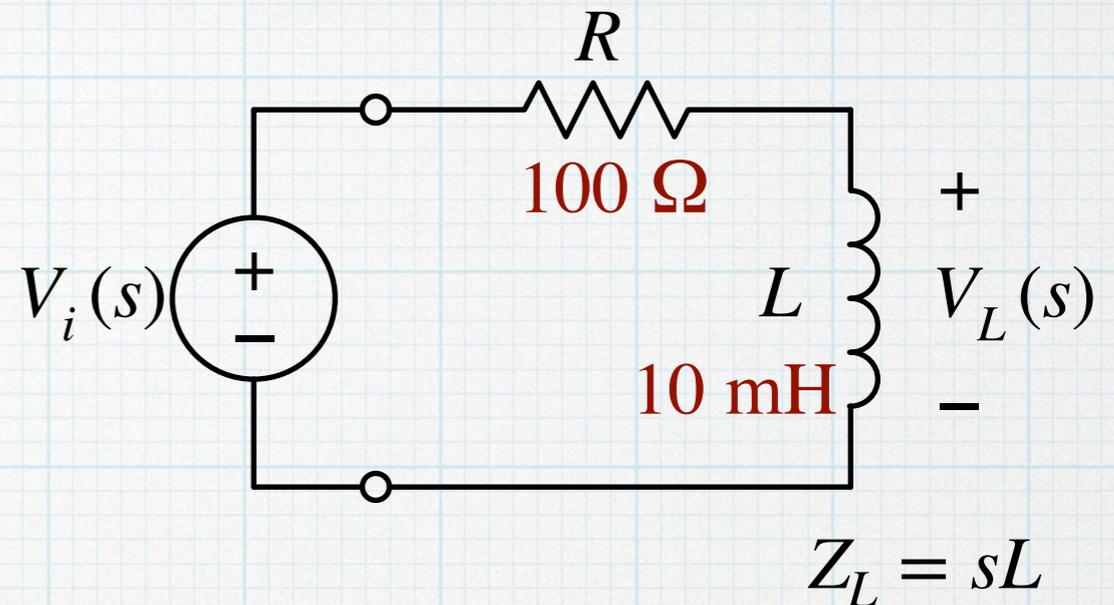
$$\text{Magnitude: } |T(j\omega)| = \frac{\omega}{\sqrt{\omega_o^2 + \omega^2}} = \frac{\omega}{\sqrt{\left(\frac{R}{L}\right)^2 + \omega^2}} = \frac{1}{\sqrt{1 + \left(\frac{R}{\omega L}\right)^2}}$$
