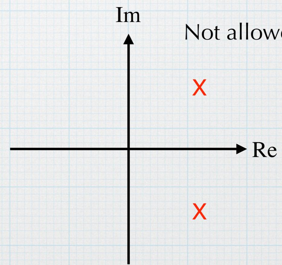
Transfer functions from circuits made with passive components — resistors, capacitors, and inductors exhibit certain characteristics.
