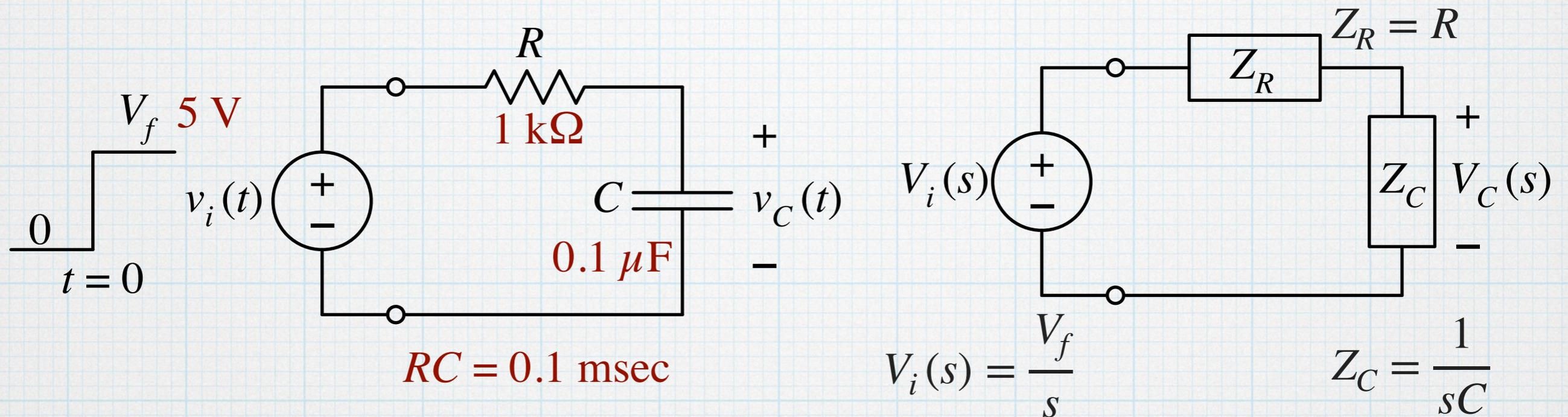
$$V_C(s) = \left( \frac{\frac{1}{RC}}{s + \frac{1}{RC}} \right) \left( \frac{V_f}{s} \right) = \frac{V_f/RC}{s \left( s + \frac{1}{RC} \right)}$$
