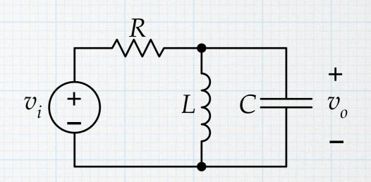
$$\omega_o = 2\pi f_o = 2\pi (3000Hz) = 18.85 \text{ krad/s}$$
