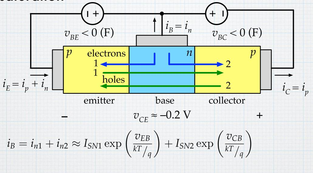
$$i_C = i_{p1} - i_{p2} - i_{n2} \approx I_{SP1} \exp\left(\frac{v_{EB}}{kT/q}\right) - [I_{SN2} + I_{SP2}] \exp\left(\frac{v_{CB}}{kT/q}\right)$$
