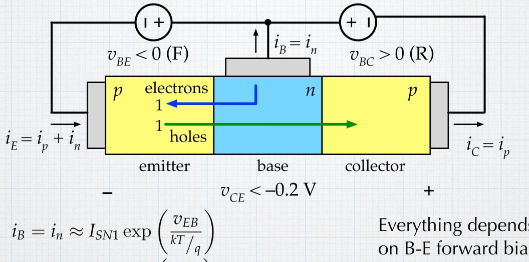
$i_C = i_p \approx I_{SP1} \exp\left(\frac{v_{EB}}{kT/a}\right)$  $i_E = i_n + i_p \approx [I_{SN1} + I_{SP1}] \exp\left(\frac{v_{EB}}{kT/a}\right)$  **Everything depends** on B-E forward bias.
