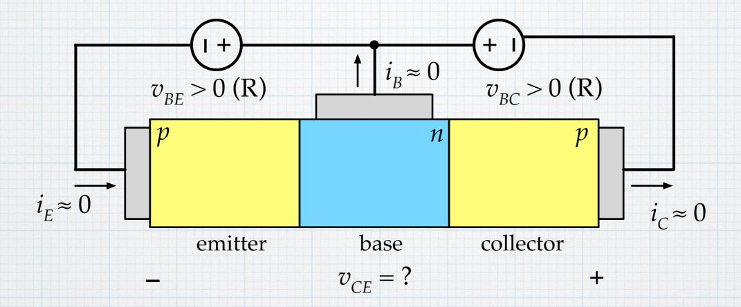
If both junctions are reverse-biased, then there are no currents (or very, very small reverse-leakage scale currents). The transistor is essentially an open circuit.
