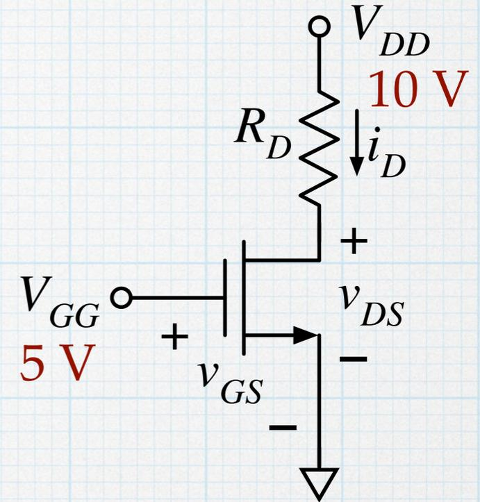
Using KVL, if  $v_{DS} = 0.2$  V, then  $v_{RD} = 9.8$  V.
