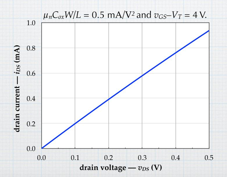
But the most important observation is that the channel resistance depends on the gate voltage! As the gate voltage is increased (which increases the electron sheet concentration in inversion layer), the channel resistance decreases. This a variable resistor. (But not anything like a potentiometer.)
