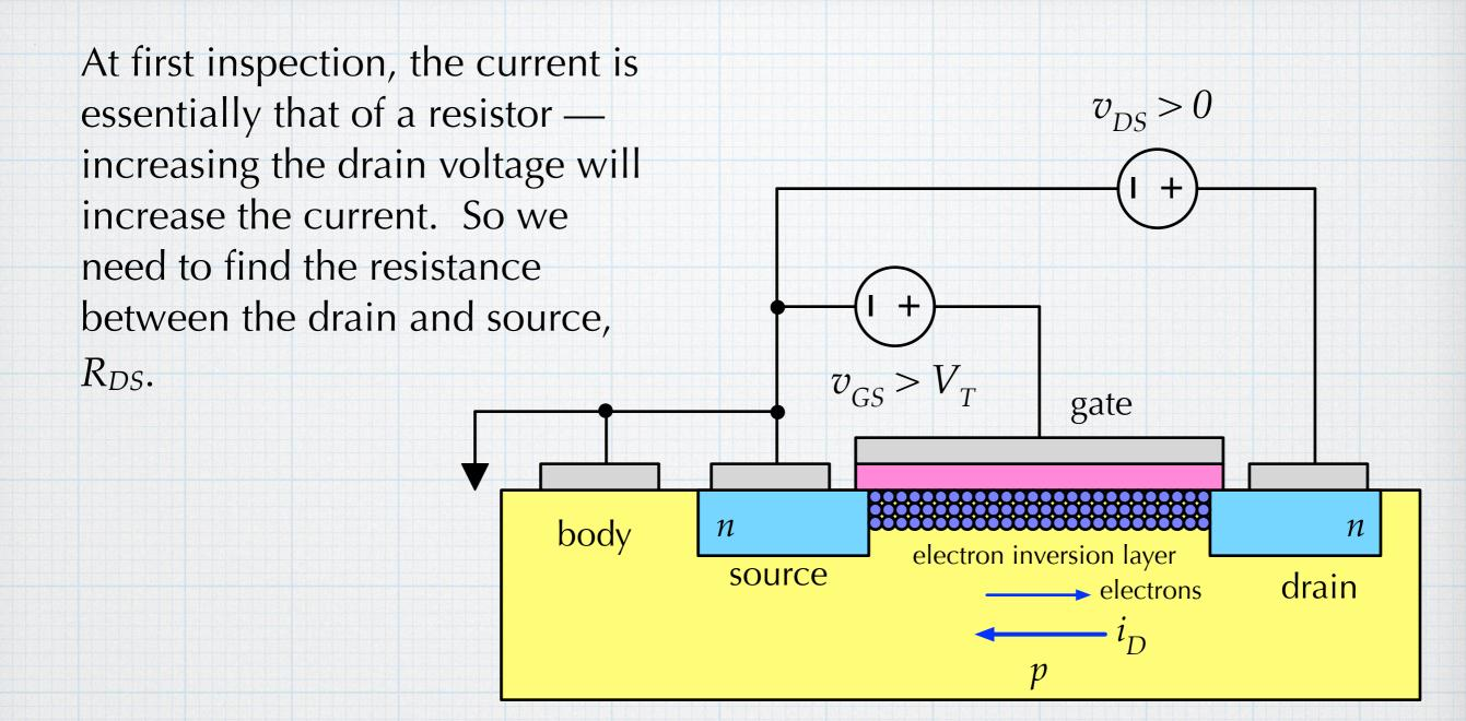
The total resistance is the sum the resistances of the three regions:  $R_{DS} = R_{source} + R_{inversion} + R_{drain}$ . Usually, the source and drain are very heavily doped (lots of electrons) and so the resistances in those regions are very small. Most of the resistance is associated with the inversion layer so that  $R_{DS} \approx R_{inversion}$ .
