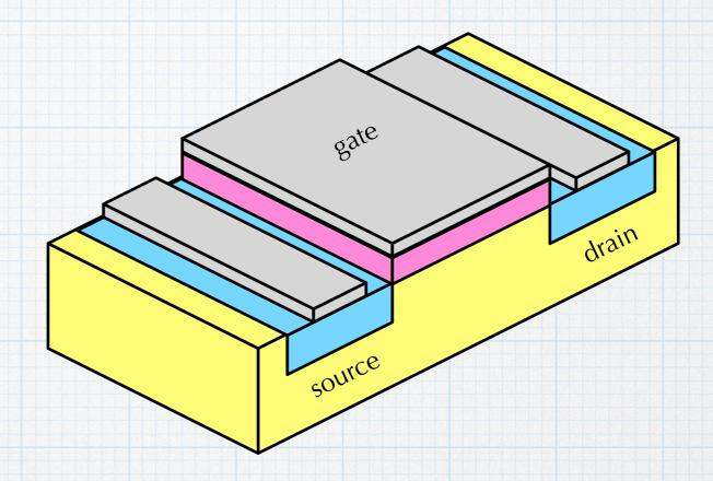
Put metal contacts on the source, drain, and oxide (gate) for electrical connection
