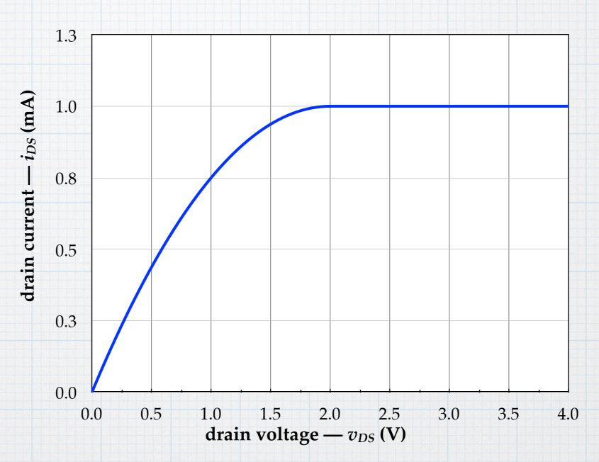
For small  $v_{DS}$  ( $v_{DS} < v_{GS} - V_T$ ), the NMOS will be in the ohmic region.
