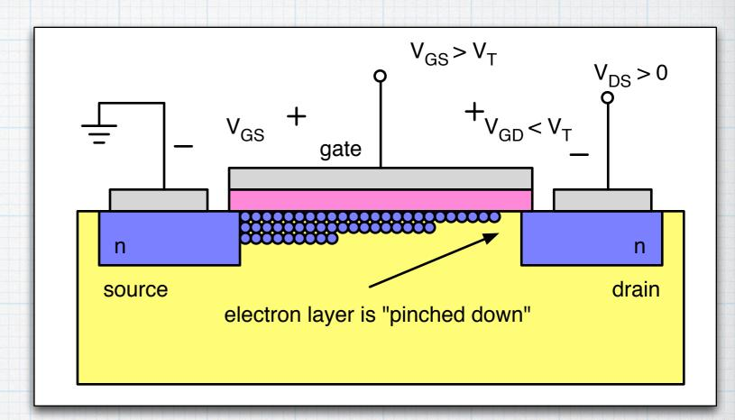
The usual terminology is to say that the channel is "pinched off" at the drain end, but this is slightly misleading. If the channel were truly pinched off, then the electron concentration would go to zero there and the current would necessarily have to go to zero, also.
