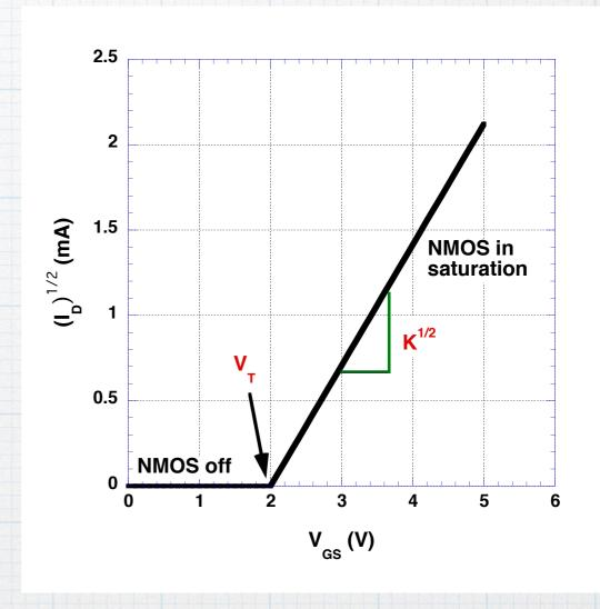
In a slight modification, we can plot  $i_D^{1/2} = K^{1/2}(v_{GS} - V_T)$ . From this graph, we can immediately pick out the two important NMOS parameters:  $V_T$  and K.
