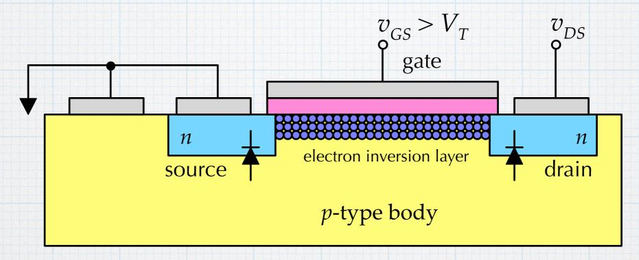
To see why, consider the p-n junctions formed by the drain and source with the substrate.
