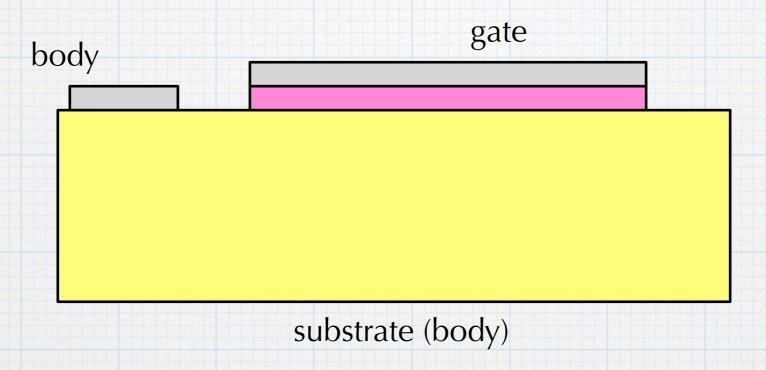
The structure is essentially a little parallel-plate capacitor formed by the gate metal and the semiconductor with the oxide as the dielectric.
