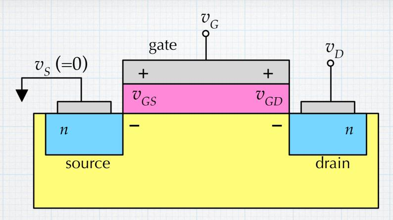
The electron sheet concentration is determined by the difference between the gate voltage and the local channel voltage. At the source end,  $qn_s = C_{ox}(v_{GS} - V_T)$ . At the drain end,  $qn_s = C_{ox}(v_{GD} - V_T)$ .
