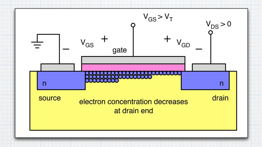
The non-uniform electron concentration along the channel implies that the channel resistance is not uniform — it is greater at the drain end, where there are fewer electrons.
