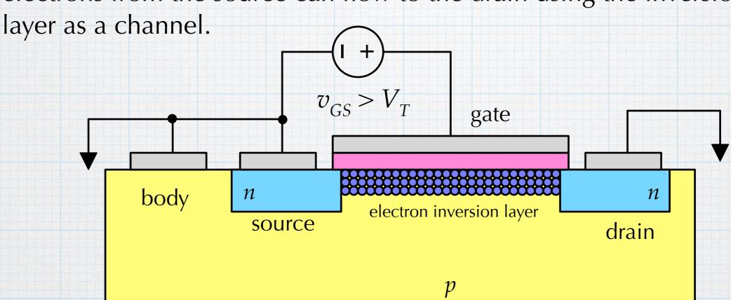
For now, we connect the source to the body (call this ground) and apply the controlling voltage between the gate and the source. This is OK for the time being, but we will have to revisit the issue of the body connection later. With the drain also at ground, the inversion layer (channel) is uniform between source and drain.
