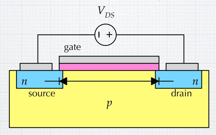
If  $V_{DS} > 0$ , the diode at the drain end will be reverse-biased, preventing current flow.
