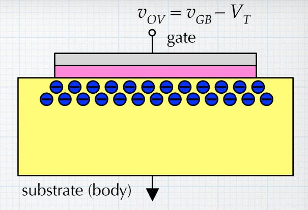
The definition of threshold is that the electron concentration under the gate is equal to the hole concentration in the rest of the substrate. If the hole concentration in the substrate is higher (due to higher doping) more voltage is required to induce the higher number of electrons needed for inversion. Increased doping means higher threshold.
