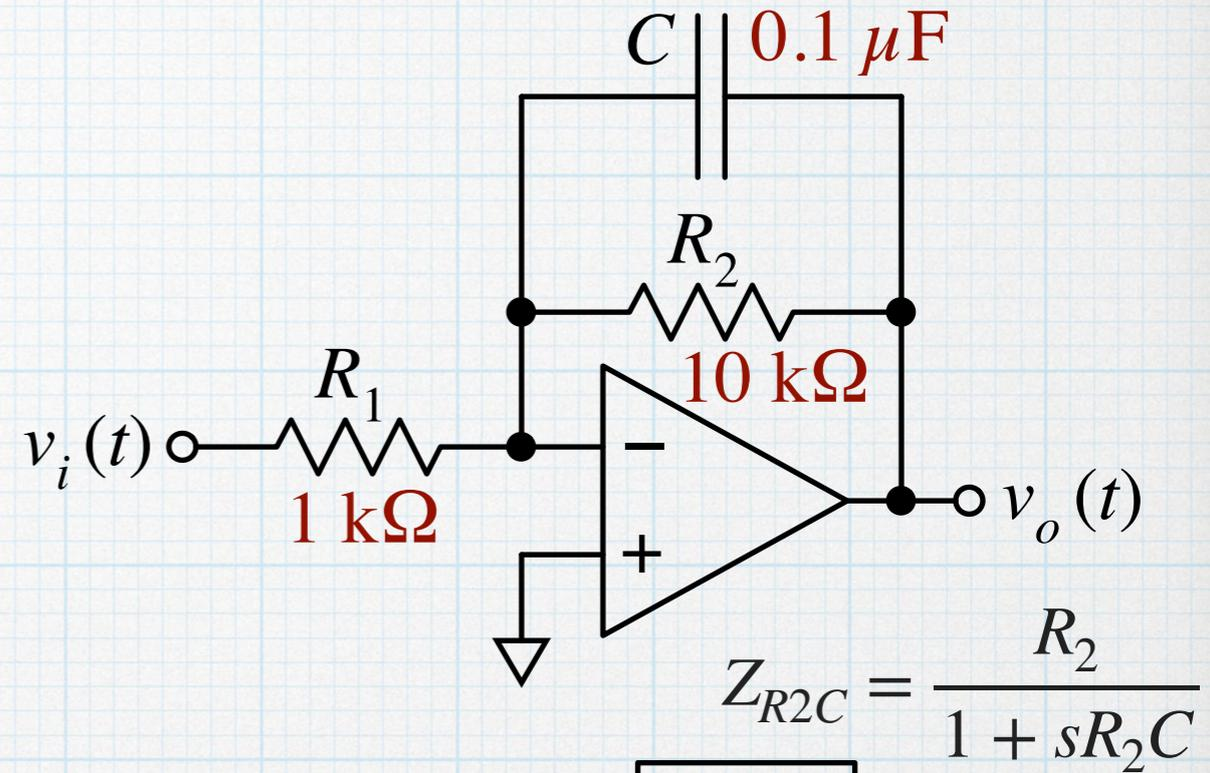
$$v_i(t) = V_A \cdot \sin(\omega t) \rightarrow V_i(s) = \frac{V_A \cdot \omega}{s^2 + \omega^2}$$
