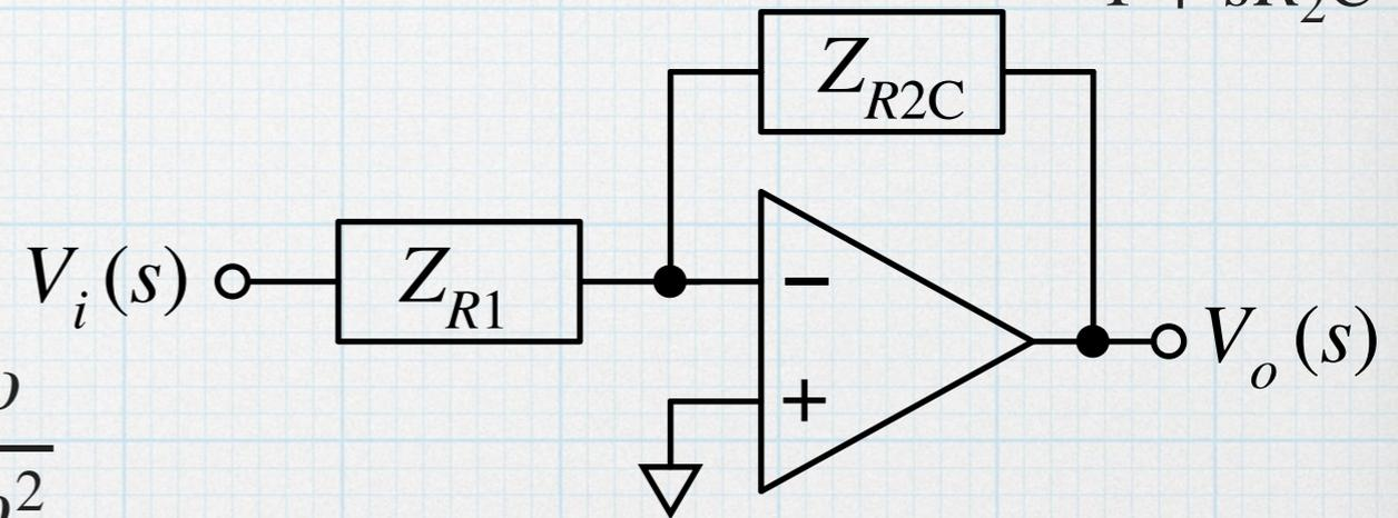
$$V_o(s) = \left( -\frac{Z_{R2C}}{Z_{R1}} \right) V_i(s) = \left( -\frac{\frac{R_2}{1 + sR_2C}}{R_1} \right) \left( \frac{V_A \cdot \omega}{s^2 + \omega^2} \right) = \frac{-\frac{V_A \omega}{R_1 C}}{\left( s + \frac{1}{R_2 C} \right) (s^2 + \omega^2)}$$
