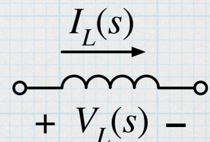
For the resistor, the frequency domain relationship is exactly the same as the the time domain. (Ohm's Law is not time-dependent, so this is not a surprise.) For the inductor and capacitor, the frequency domain relations are actually simpler. All three components can be treated with a simple "Ohm's-Law-like" current-voltage equation:
