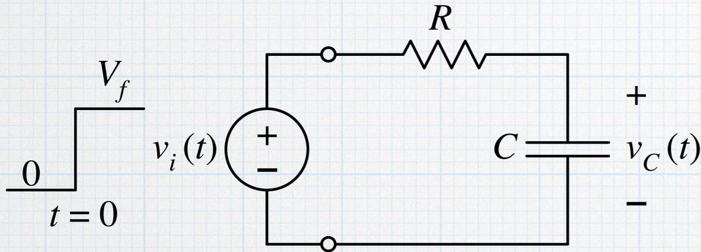
The frequency domain circuit is easily solved using a voltage divider.
