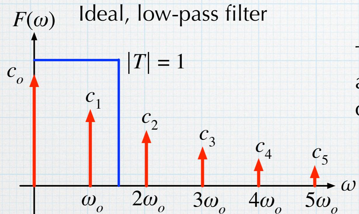
The signal components at  $c_o$  and  $c_1$  pass through. All higher order components are cut-off.
