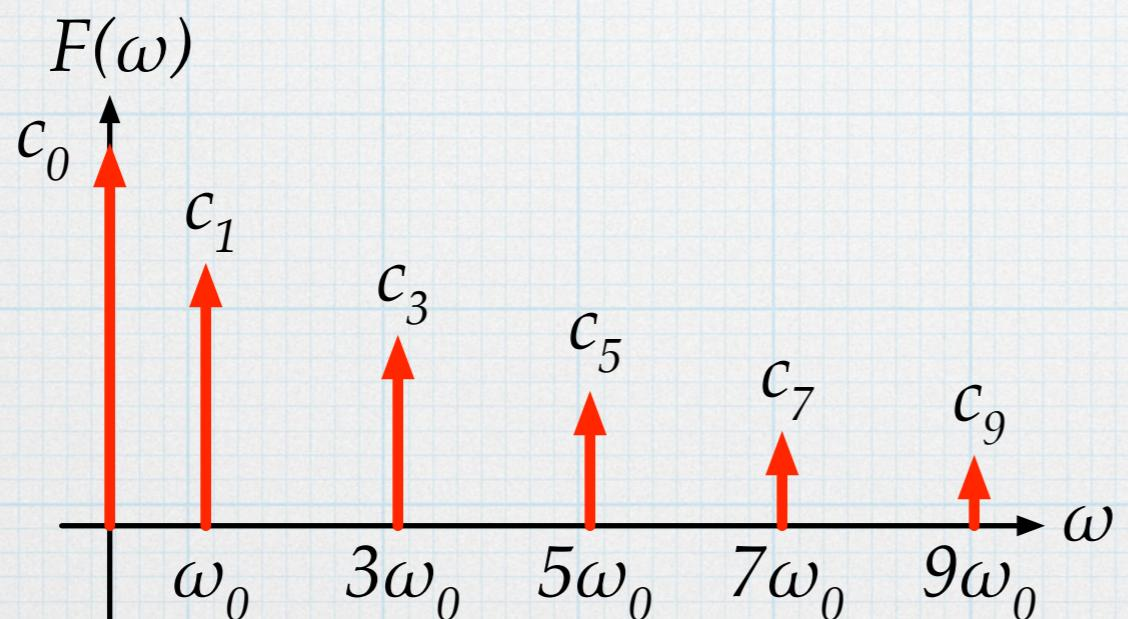
What happens when we apply a sinusoidal signal to a filter. The Fourier series line spectrum shows us exactly what will happen. Consider a low-pass filter. (Make it ideal, just for simplicity.)
