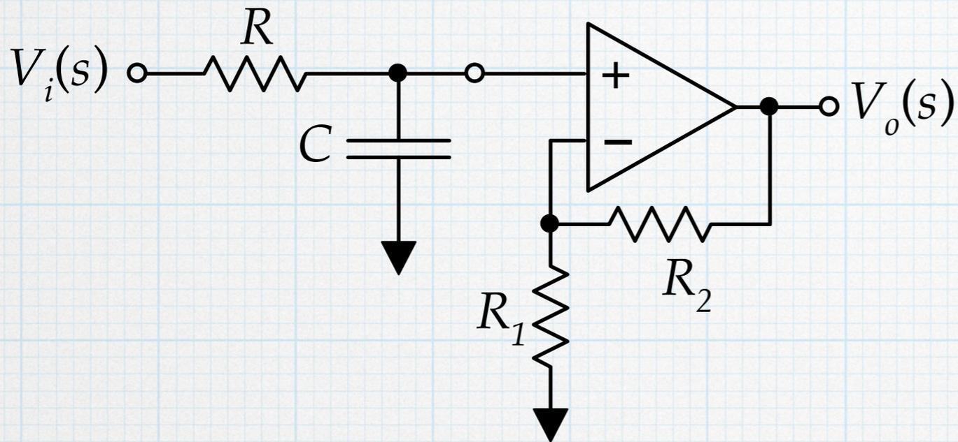
Note: It might slightly disingenuous to treat this as if it were some new type of filter — we can readily see that it is a simple RC filter cascaded with a simple non-inverting amp. However, it is still a useful circuit.
