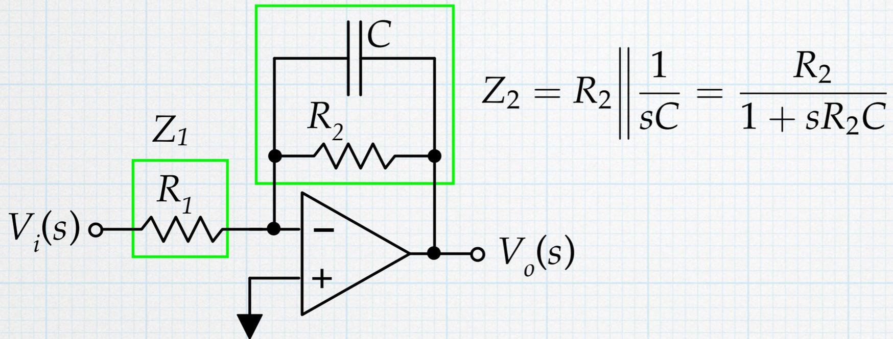
$$T(s) = \frac{V_o(s)}{V_i(s)} = -\frac{Z_2}{Z_1} = -\frac{\frac{R_2}{1+sR_2C}}{R_1} = \frac{-\frac{R_2}{R_1}}{1+sR_2C} = \left(-\frac{R_2}{R_1}\right) \frac{\frac{1}{R_2C}}{s + \frac{1}{R_2C}}$$
