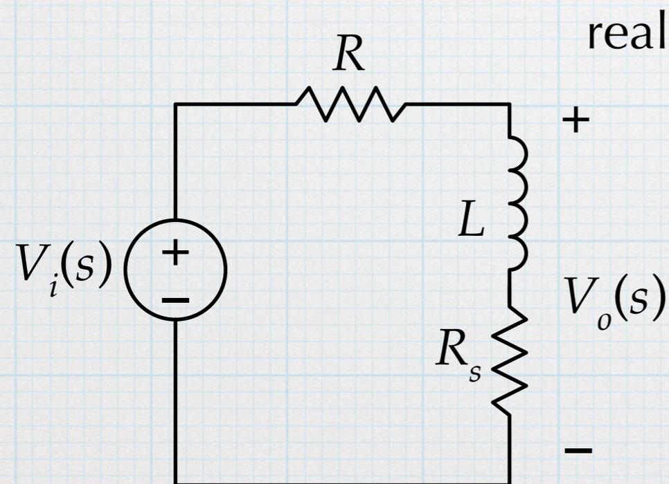
$$T(s) = \frac{sL + R_s}{sL + R_s + R_1} = \frac{s + \frac{R_s}{L}}{s + \frac{R_s + R_1}{L}} = \frac{s + \omega_Z}{s + \omega_P}$$
