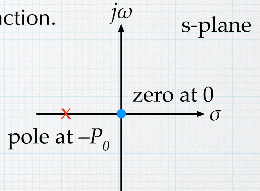
We will ignore the gain initially (set  $G_o = 1$ ) and focus on sinusoidal behavior by letting  $s = j\omega$ .
