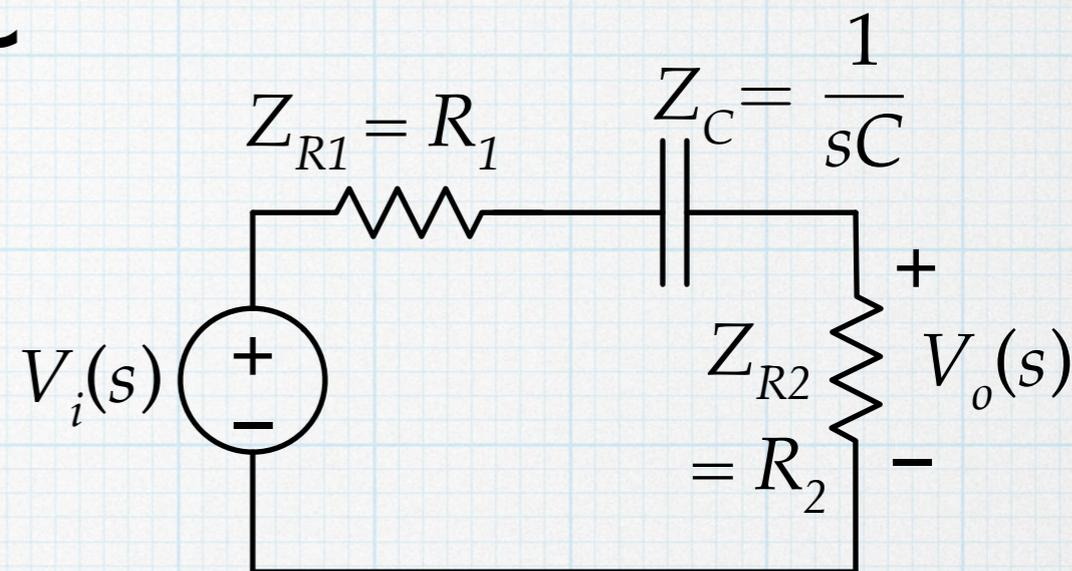
$$G_o = \frac{R_2}{R_1 + R_2} \quad \text{Note the voltage divider. "Gain" } < 1.$$
