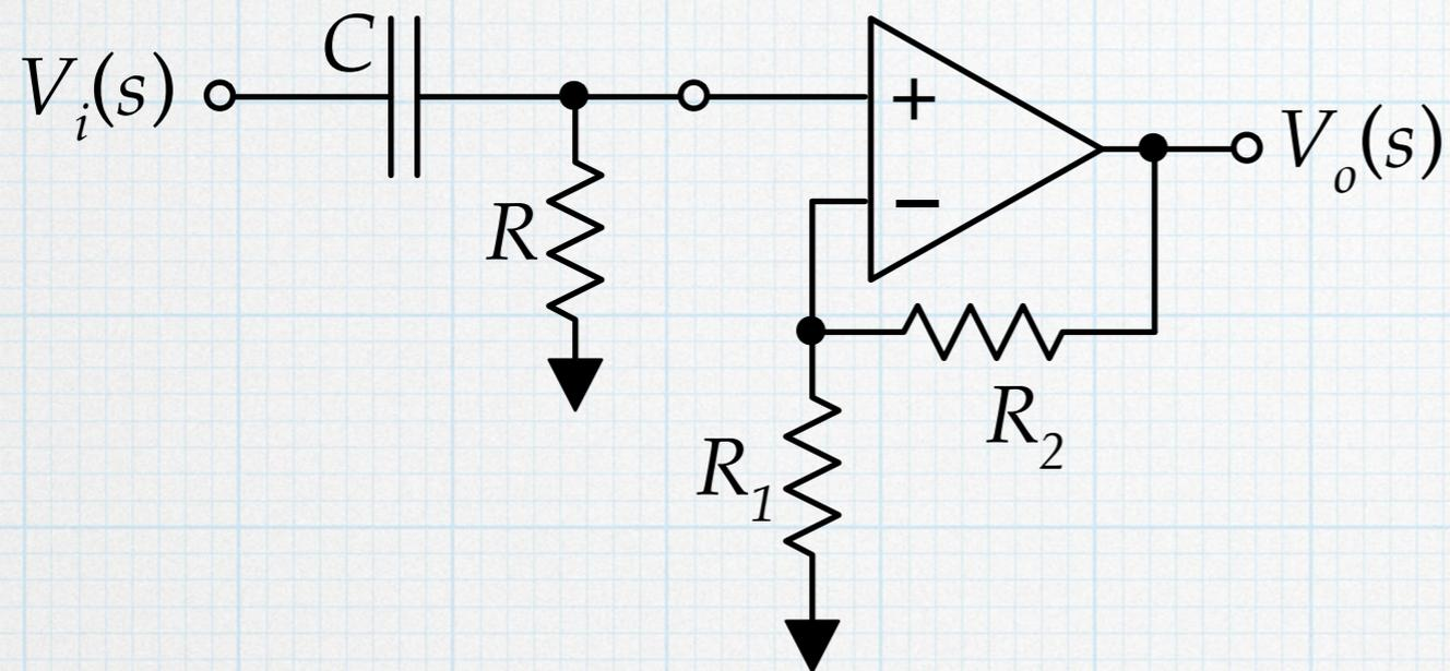
Again, this is simple  $RC$  high-pass cascaded with a non-inverting amp.
