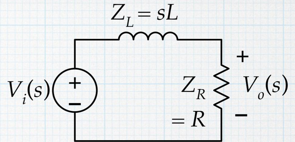
Use a voltage divider to find the transfer function.
