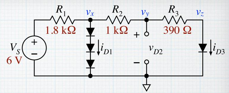
As  $R_1$  increases, the current available from the source decreases. At some value of  $R_1$ , the available current is not sufficient to keep all the diodes on. Some will have to turn off to balance the current — in this case, the middle string is off. So try again, this time with the the  $D_2$  string off.
