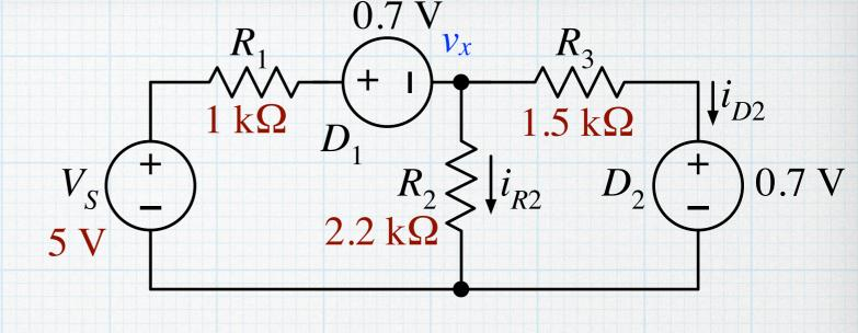
Inserting values, we arrive at  $v_x = 2.25 \text{ V}$ .
