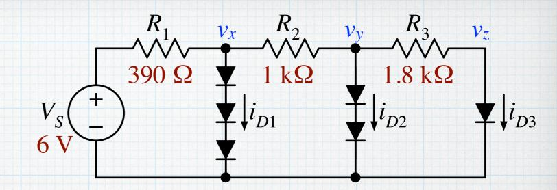
When diodes are in series, there must be sufficient voltage to turn on all of the diodes in the string — if one diode in the string is off, there can be no current and effectively all of them are off. If the 3-diode string is on, then the total voltage across it must be  $3 \cdot (0.7 \text{ V}) = 2.1 \text{ V}$ . Similarly, the 2-diode string must have 1.4 V across for current to flow.
