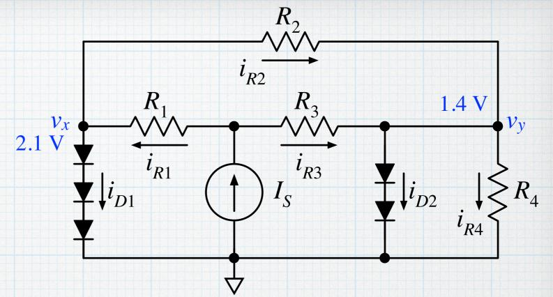
These are two equations in two unknowns —  $i_{R1}$  and  $i_{R3}$  — and can be solved in a straight-forward manner to give:  $i_{R1} = 5$  mA, and  $i_{R3} = 5$  mA.
