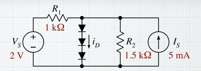
The source voltage by itself is insufficient to forward-bias the the diodes. (Need 2.1 V across diodes.) What effect does the current source have? It could certainly supply current to the diodes. Let's roll the dice and assume the the diodes are off. If true, the answer is trivial —  $i_D = 0$ . We need to check, though. The reduced circuit reduces to a familiar one from EE 201.
