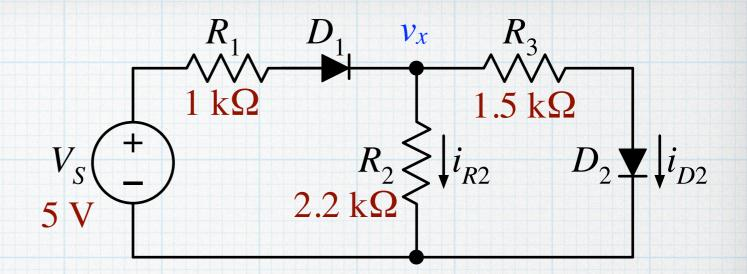
We can be fairly certain, given the polarity of the source, that  $D_1$  will on. (If it weren't, then all of the source voltage would appear across the diode as a positive voltage — an obvious contradiction. If it's not obvious, write a KVL equation around the left-hand loop and set the current to 0.)
