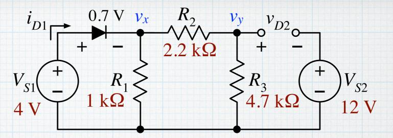
The right-hand source is disconnected by the reverse-biased  $D_2$ . What's left are  $V_{S1}$ ,  $D_1$ , and the equivalent resistance of  $R_1$  in parallel with the series combination of  $R_2$  and  $R_3$ . This is "201-easy".
