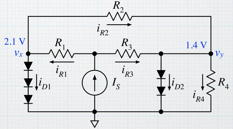
However, the on/off nature of the diodes make this problem more tractable. Start with assumptions — it looks like the current from the source would split and flow through the diode strings. So, let's assume that all diodes are on. Then we know two of the node voltages, as indicated.
