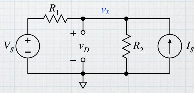
Inserting values and calculating:  $v_x = 4.20 \text{ V} \rightarrow \text{way bigger than } 2.1 \text{ V}$ . The diodes must be on. So try again.
