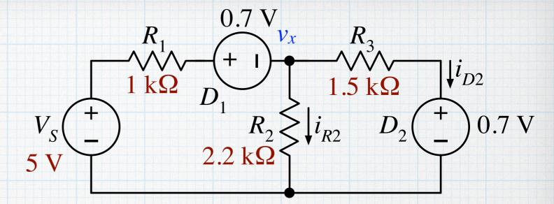
As we will see in these examples, the diodes, when treated as being either on or off, can make the analysis simpler. Sometimes we will need to be a little bit clever and use "super-node" ideas, but even then, the problems are usually not too hard. For example, in the circuit above, we note that the voltage across  $R_1$  is  $v_{R1} = V_S - (v_x + 0.7 \text{ V})$  and the voltage across  $R_3$  is  $v_{R3} = v_x - 0.7 \text{ V}$
