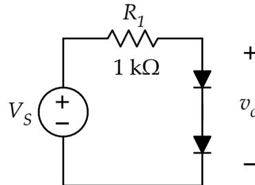
Finally, limit both the positive and negative of the source using the circuit of Fig. 7. Observe the input and output together on the oscilloscope, and record a copy of the trace for your report.
