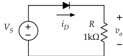
Figure 1. Half-wave rectifier.
