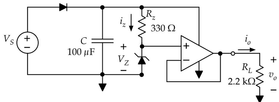
The op-amp is in the unity-gain configuration, so the output voltage should be equal to the Zener voltage.
