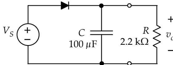
Use the cursors on the oscilloscope to measure the ripple voltage  $[v_o(\text{max}) - v_o(\text{min})]$ . Use the multimeter on the DC voltage setting to measure the average output voltage. Compare these measured ripple and average voltage to calculated values, using the equations derived in class (or in the book).
