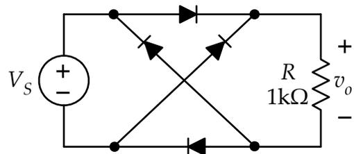
Figure 2. Full-wave rectifier.
