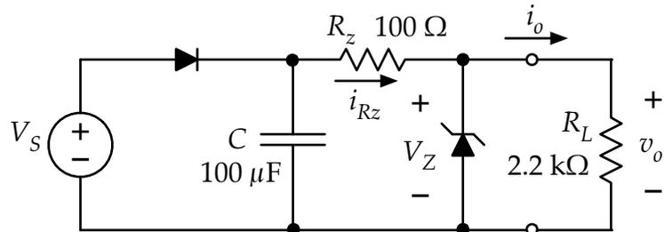
Repeat all the measurements from part C. (Different load resistance and different source amplitudes.) Note that it may be difficult to measure the ripple voltage using the oscilloscope, because the ripple should be much smaller. (Of course, this is the point in using the regulator circuit.) Record the ripple and the average voltages measured using the meter.
