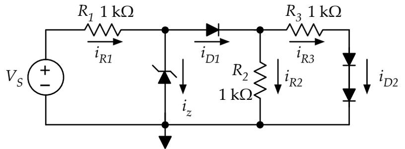
Figure 7. Find the all of the indicated currents. Do this first for  $V_S = +8$  V, and then repeat for  $V_S = +12$  V.
