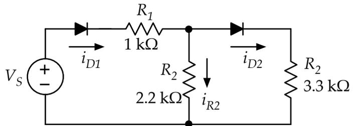
Figure 3. Do this first with  $V_S = +5$  V. Then repeat with  $V_S = -5$  V.
