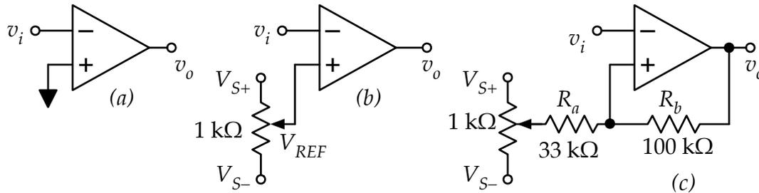
Subtle detail: In the feedback network of part (c),  $R_a$  actually consists of the 33 kΩ fixed resistor plus the Thevenin equivalent resistance of the 1-kΩ potentiometer (parallel combination of the two arms of the potentiometer). However, the Thevenin resistance is small – no bigger than 500 Ω – and so you can reasonably ignore it in comparison to the 33-kΩ resistor.)
