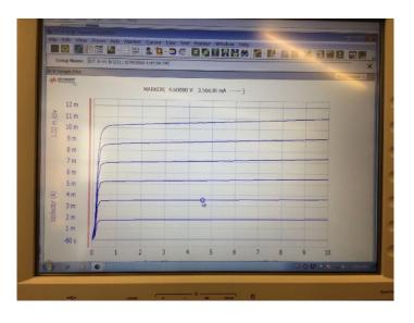
The marker is on the second of the family of curves, which in this case corresponds to a base current of 20  $\mu$ A. The collector current at the marker is 3.566 mA.
