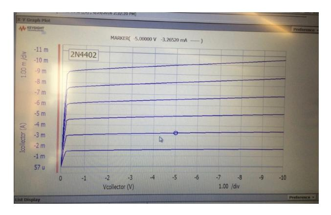
The above plot was obtained for a 2N4402 *pnp* transistor (similar to the 2N2907 that is in your lab kit.) Note the negative values on the voltage and current axes. The curves correspond to base currents ranging from  $-10 \,\mu\text{A}$  to  $-60 \,\mu\text{A}$ . From the marker coordinates, we can determine the current gain for the transistor to be  $\beta_F = (-3.265 \,\text{mA}) / (-20 \,\mu\text{A}) = 163.3$ .
