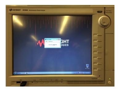
3. Once EasyEXPERT is running, begin the setup by choosing the "Discrete" category (meaning discrete component measurements) and then the specific BJT Ic-Vc Ib measurement from the Discrete library.
