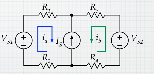
Define the voltages for the components around each mesh and write KVL equations.
