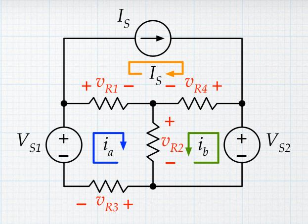
Use Ohm's law to write the resistor voltages in terms of the mesh currents. It is important to pay attention to current directions and voltage polarities.
