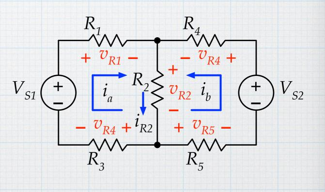
We can write the resistor voltages in the two equations in terms of the currents, using Ohm's law. Recall that  $i_{R2} = i_a + i_b$
