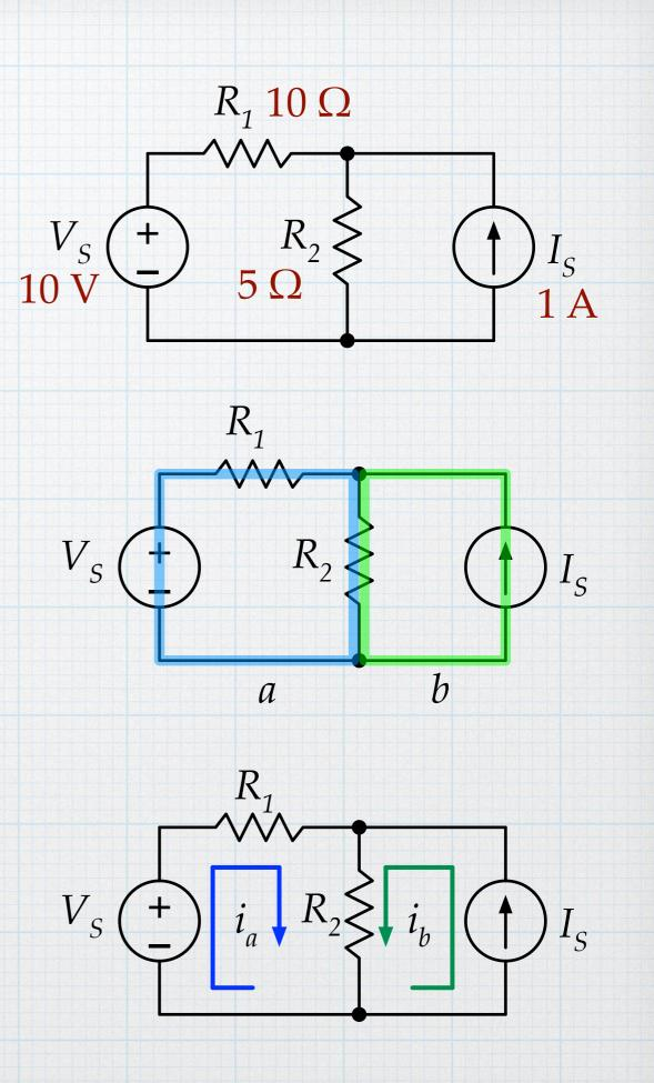
We note something interesting in this case — loop *b* has a current source in an outside branch. Therefore,  $i_b$  must be equal to  $I_s$ . We won't need to solve for  $i_b$ because we already know it. Also, we see that  $i_{VS} = i_{R1} = i_a$  and  $i_{R2} = i_a + i_b = i_a + I_s$ .
