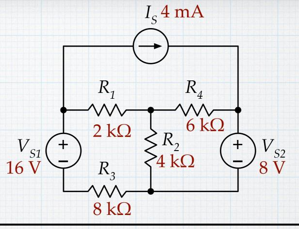
We will need to find  $i_{VS1} = I_S + i_{R1}$ . The resistor  $R_3$  on the bottom would make the use of node voltages a bit unwieldy, so try mesh currents.
