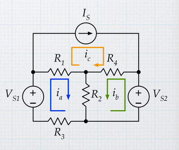
With the current source in the outside branch of mesh c, we know directly that  $i_c = I_s$ . That leaves two unknown mesh currents.
