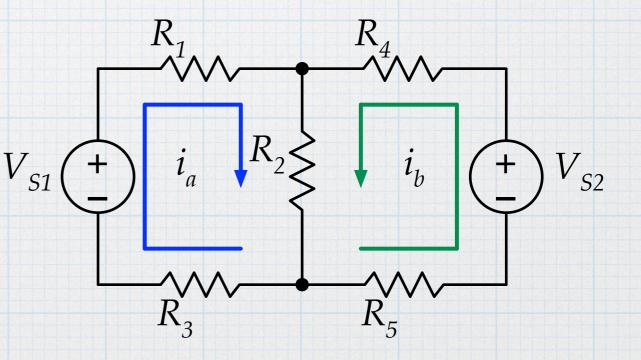
Identify the voltage drops on each component. Make sure that the resistor polarities are commensurate with the directions of the mesh currents.
