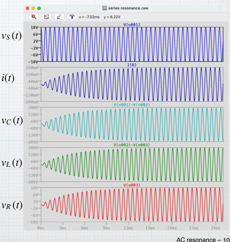
If the resistance is increased, say to  $R = 5 \text{ k}\Omega$ , so that the transient is no longer underdamped, we still see resonance,  $v_R = v_S$  and  $v_C = -v_L$ .
