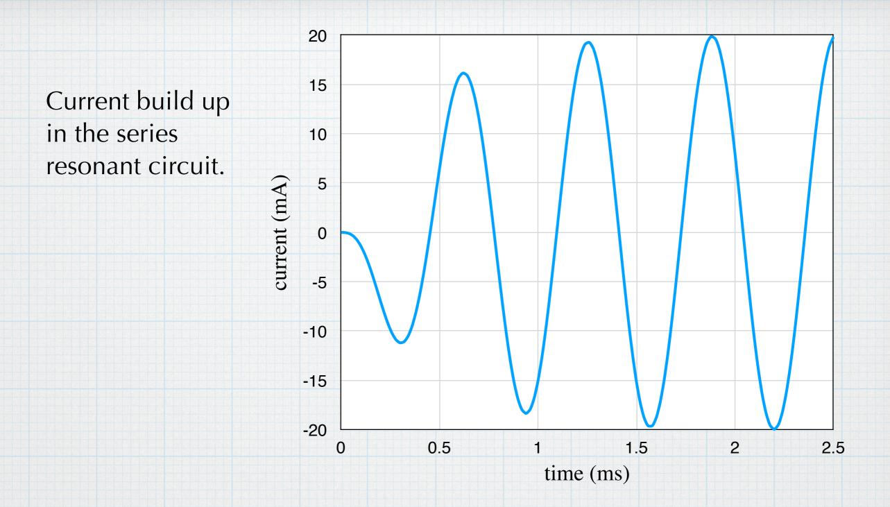
At the start the current is small, but it builds up with each cycle. With a time constant of 0.4 ms, the transient is essentially complete by 2 ms. After that, the current oscillates at the source frequency (which is the resonant frequency of the circuit), with an amplitude of 20 mA, corresponding to the resistor voltage of 10 V and inductor and capacitor voltages of 20 V.
