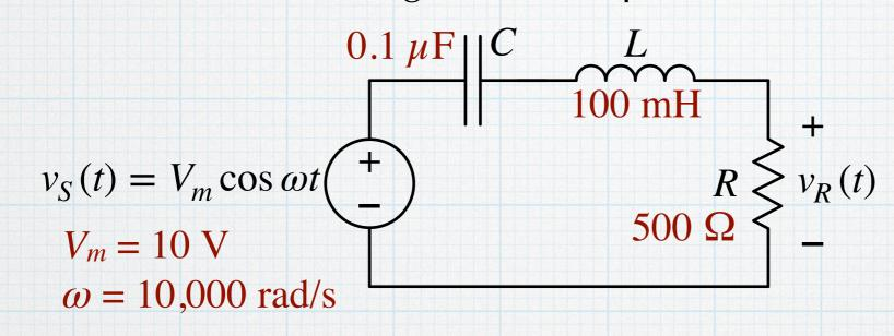
The complex voltage on the resistor is easily found using a voltage divider with the three impedances:  $Z_C$ ,  $Z_L$ , and  $Z_R$ .
