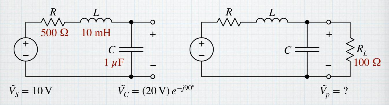
We immediately see the problem as we start the AC analysis. The extra resistor changes the impedance:
