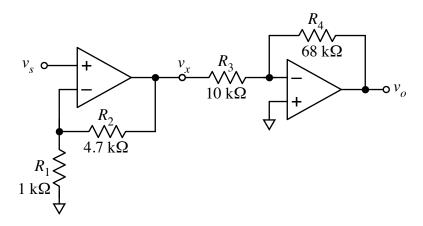
For  $v_s$ , use the function generator set to a sinusoid with frequency of 1000 Hz and amplitude of 0.25 V<sub>RMS</sub>.
